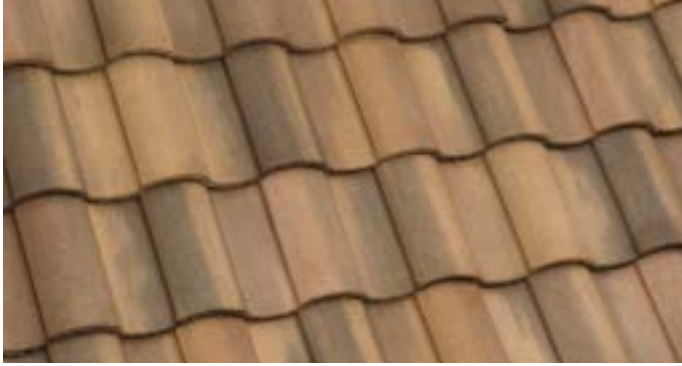
3814 San Pablo Blend - Blend of Golden Tan, Terracotta, Medium Brown, W/Streaks CRRC 0918-0092 Ref. .23 Emi. .93 Sri 24 A.Ref. .24 A.Emi. .95 A.Sri 26
